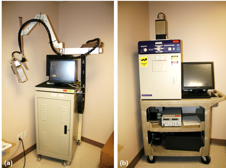
Fig. 2. Image of (a) the intraoperative imaging system used to assess lymphatic drainage of the arm and breast in the operating suite and (b) the ex vivo imaging system to assess the fluorescent status of the excised lymph nodes in the pathology suite.
