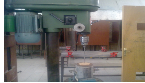
FIGURE 2: A view of performing a hole with drill along the longitudinal axis of compacted sample.
