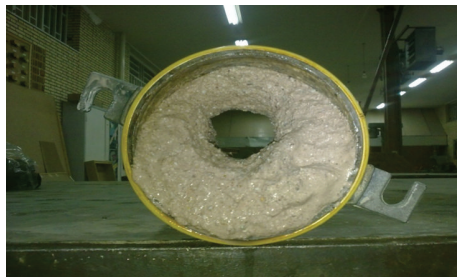
FIGURE 8: The hole size of unstabilized soil after performing the hole erosion test.
