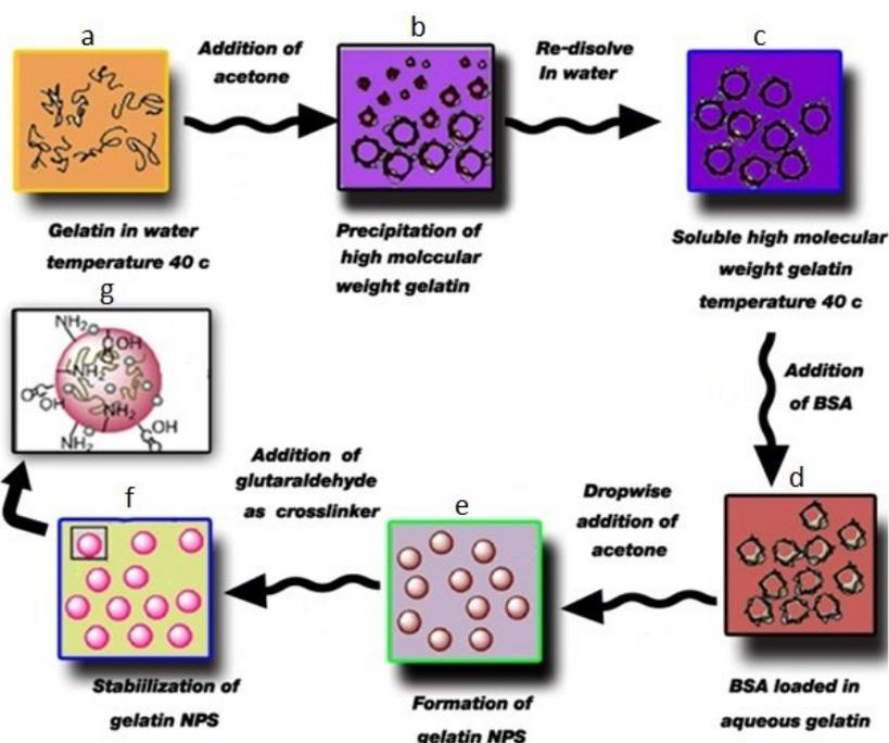
**Fig. 1.** Schematic illustration of BSA-loaded gelatin nanoparticles produced by two-step desolvation. (a) Aqueous solution of gelatin; (b), first step desolvation; (c), aqueous solution of high molecular weight of gelatin; (d), BSA- loaded in aqueous gelatin; (e), dropwise addition of acetone and formation of GNP, and (f), stabilization of GNP by glutaraldehyde [19].
