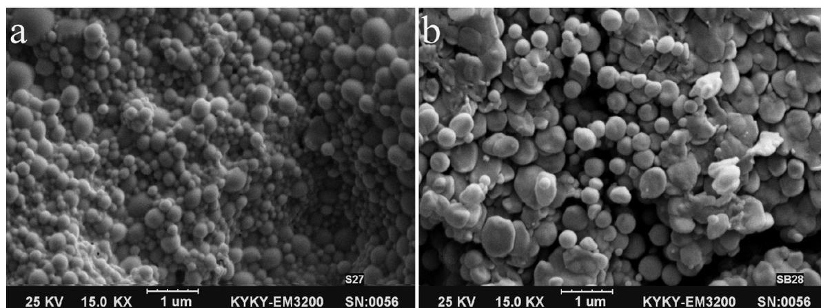
**Fig. 4.** Scanning electron microscopy images of gelatin nanoparticles (1- $\mu$ m scale). (a) Gelatin nanoparticles with 2% w/w BSA, (b) gelatin nanoparticles with 3% w/w BSA fabricated by two-step desolvation method.
