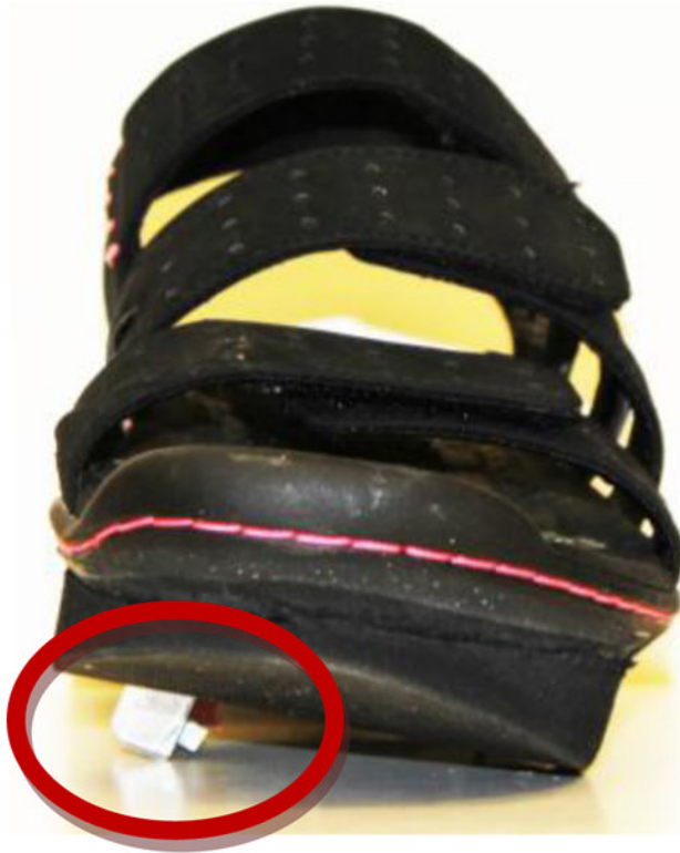
Figure 1. Picture of the perturbing shoe Anterior view of the sandal, unloaded by body weight and with the 18.4mm-high lateral flap (circled) deployed in the parasagittal plane so as to invert the foot during a single mid stance phase
