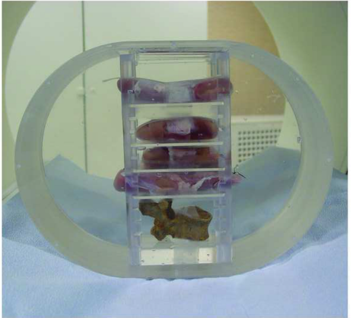
Fig. 2. Photographs show a porcine kidney that has renal stones sutured inside (a) and the set up of the water phantom (b). Stone-filled kidneys were placed in a 35cm water phantom anterior to a cadaver spine to create realistic scattering and attenuation conditions (b).
