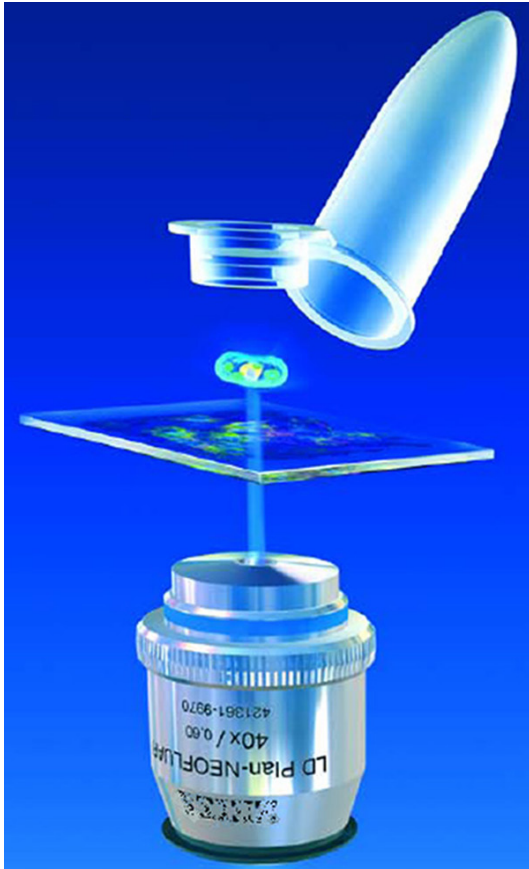
Figure 3. Catapulting of a selected tissue region into the cap of a conventional tube containing a few microliters of extraction buffer (Copyright by http://www.zeiss.com ).
