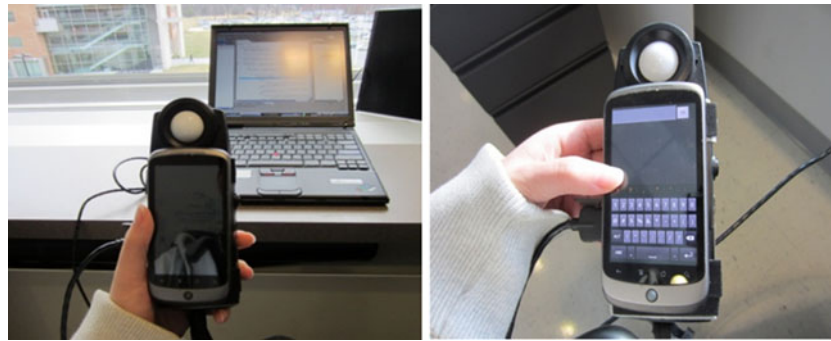
Fig. 3 Experimental setup. The handheld device was attached to the face of the T-10 such that the sensor was able to capture illuminance readings of the background. The T-10 was connected to a laptop computer through a proprietary RS232 cable because due to Android OS limitations, the handheld devices were not able to directly interface with the T-10. The T-
