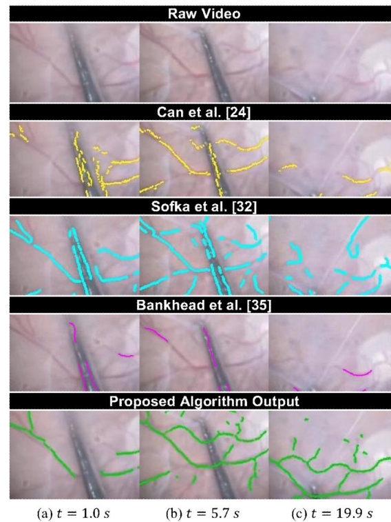
Fig. 5. Comparison of our approach (30 Hz) to the vessel detection algorithms of Can et al. [24] (80 Hz), Sofka et al. [32] (0.3 Hz), and Bankhead et al. [35] (8 Hz) on a 20 s video of human retina during an in vivo membrane peel. Source: http://youtu.be/_naooJFuxPI
