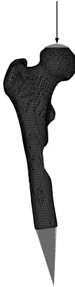
Figure 1. Anterior view of the FE-model, generated from a QCT scan. Displacement was applied to the model via the cup on the head of the femur, while the bottom of the model was fixated by means of high stiffness springs.
