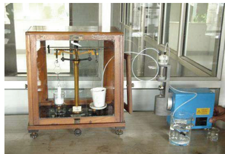
FIGURE 1: Modified two pan balance used for in vitro mucoadhesion studies.
