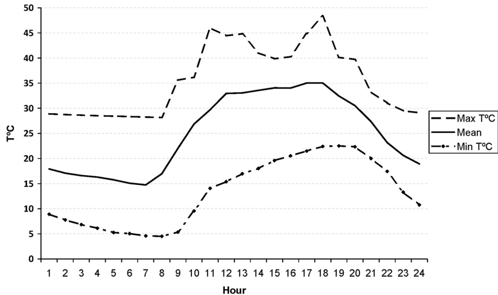
FIG 2 Maximum and minimum hourly temperatures (T) and average temperatures recorded by the data loggers from 6 July 2012 to 6 September 2012. Temperatures reached a maximum of 48°C at 6:00 p.m. and a minimum of 4.52°C at 8:00 a.m. The average for the 2 months was 21.97°C.
