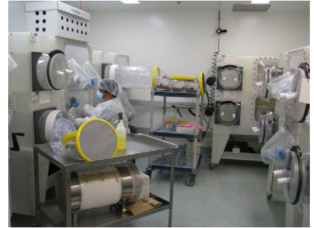
Germ-free enclosures house mice for gnotobiotic research. Image courtesy of the National Institute of Allergy and Infectious Diseases.
