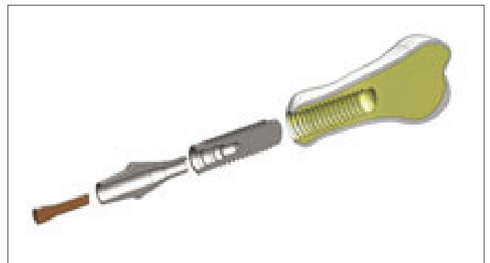
[Table/Fig-1]: The 3D CAD finger bone model containing cortical bone and cancellous bone along with prosthesis system was made
