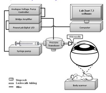
Figure 1. Schematic diagram of experimental setup for feedback-coupled, single-needle, constant-pressure, anterior chamber perfusion in live mice. A 35-G needle for anterior chamber cannulation was connected via a rigid tube to a pressure transducer then to a microsyringe pump, bridge amplifier, and digital input/output (I/O) unit integrated with analytic software on a computer. The pump controller provided a feedback loop between the pressure transducer and the pump and amplifier.
