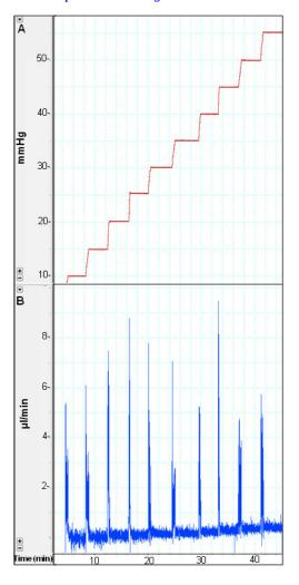
Figure 2. Example of pressure and flow rate traces for constant-pressure perfusion at pressures of 10-55 mmHg. **A**: Pressure (y-axis; scale 5 mmHg per square) versus time (x-axis; scale 2 min per square); **B**: flow rate (y-axis; scale 1  $\mu$ l/min per square) versus time (x-axis). Spikes in the flow trace reflected a momentary increase in flow rate as the pump sped up. Flow rates then automatically readjusted to a lower steady rate commensurate with the new set-point pressure.
