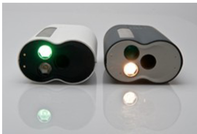
FIGURE 2. The Gynocular showing lens, green filter, and warm white LED illumination.
