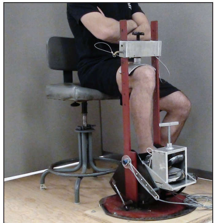
Figure 5. Boot apparatus for measuring the maximal voluntary contraction with the plantar flexors.
