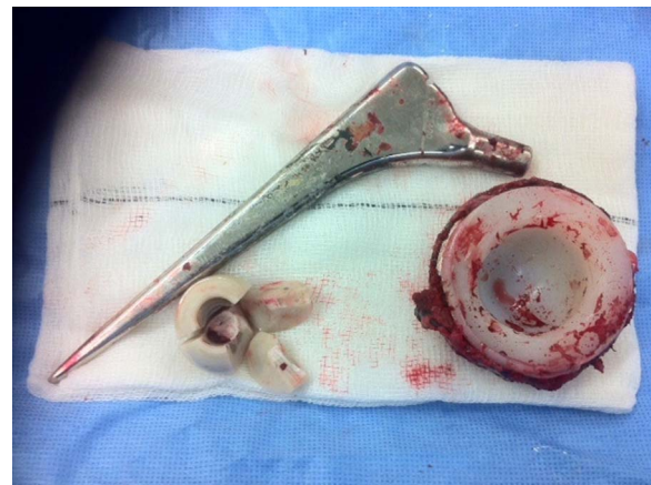
Figure 3 The explanted implants including the femoral stem, polyethylene acetabular liner and fractured ceramic femoral head.
