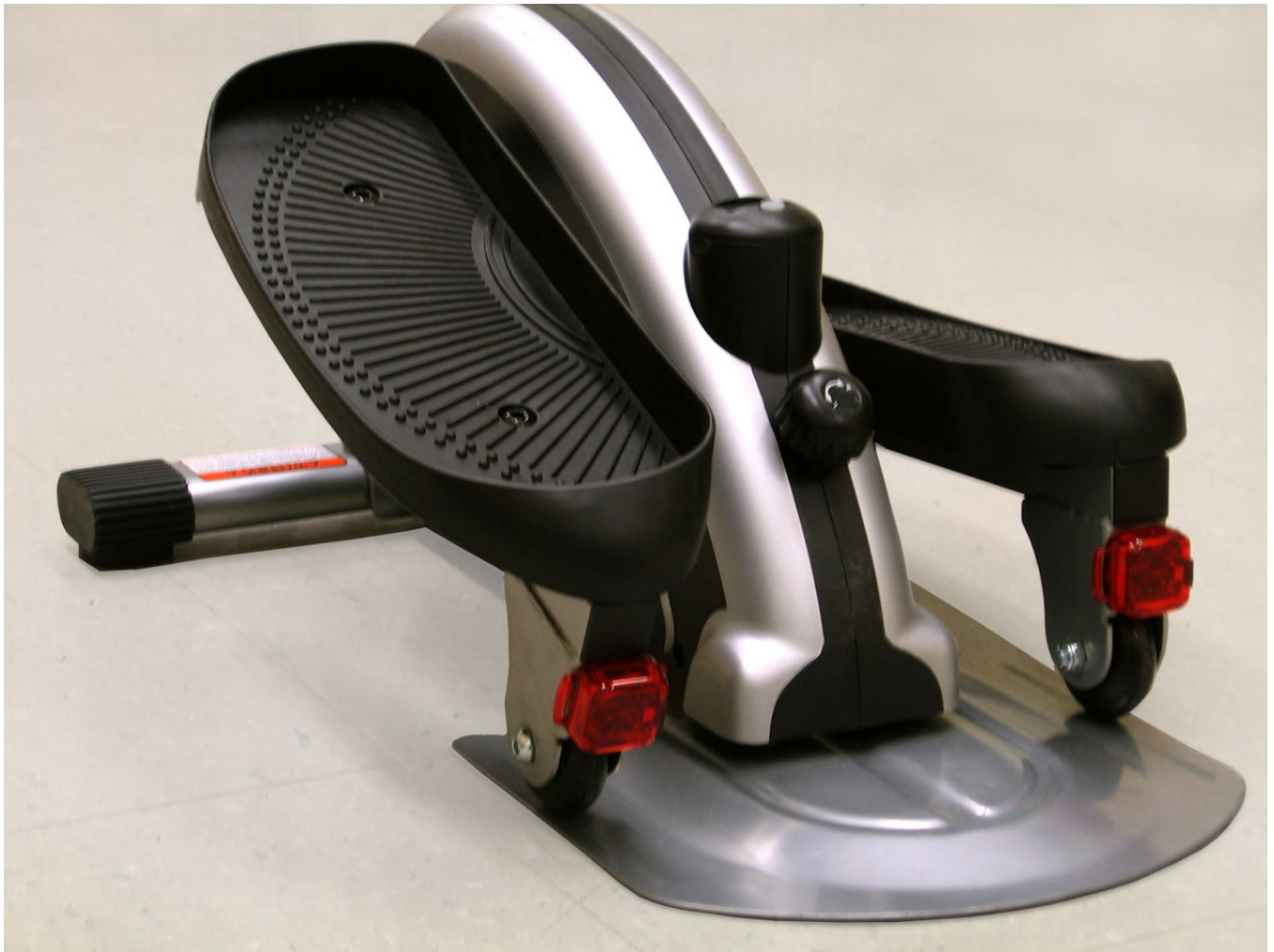
Figure 1. Compact elliptical device with accelerometers attached at rear of each foot pod.
