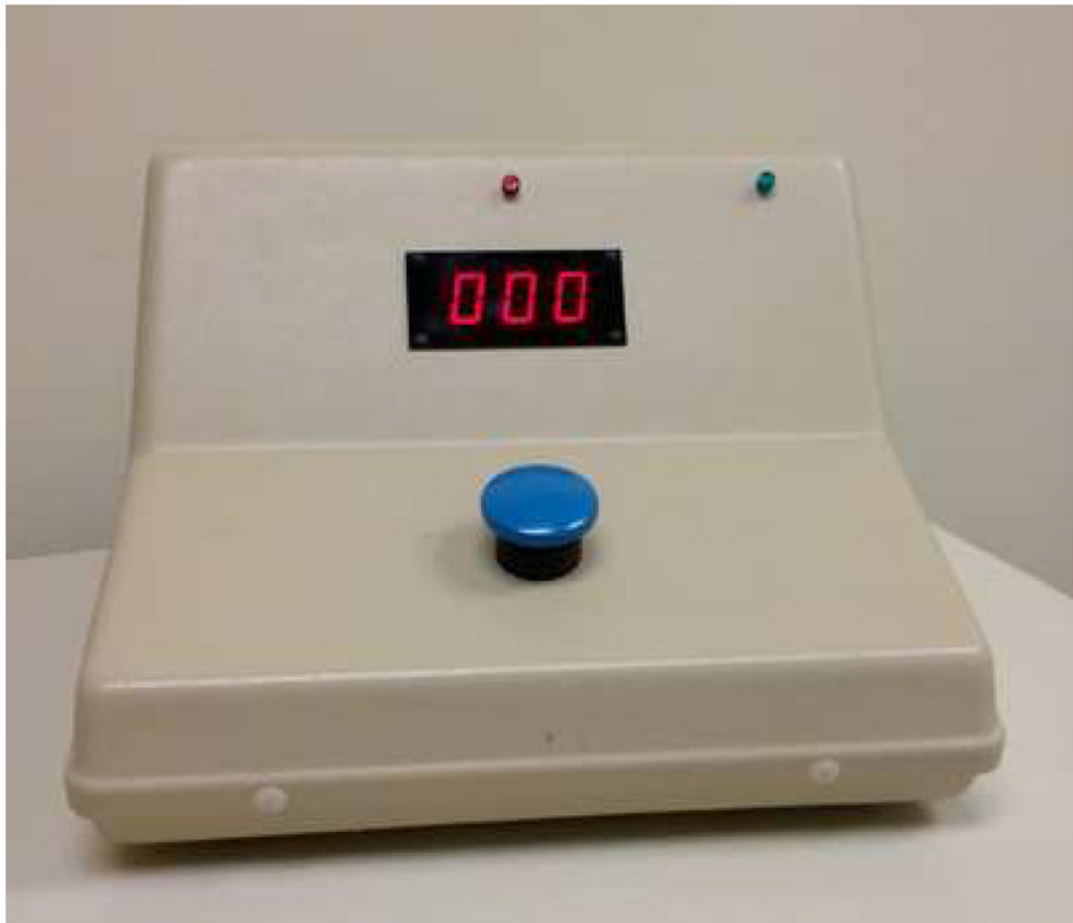
Figure 1. The Gordon Diagnostic System has an LED display upon which stimuli are presented, and a large blue button for making responses. The red and green lights do not provide feedback on performance, but only indicate whether a data collection session is ready to proceed or has terminated.
