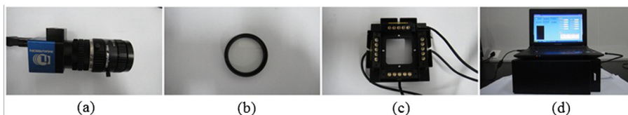
Figure 6 Hardware units of the device. (a) CCD image sensor. (b) UV filter. (c) Excitation light source. (d) Integrated instrument.
