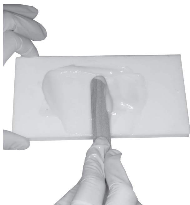
Figure 2- Homogeneous paste of castor oil polyurethane (COP) obtained after manual mixing and mixing with a spatula on a Teflon plate
