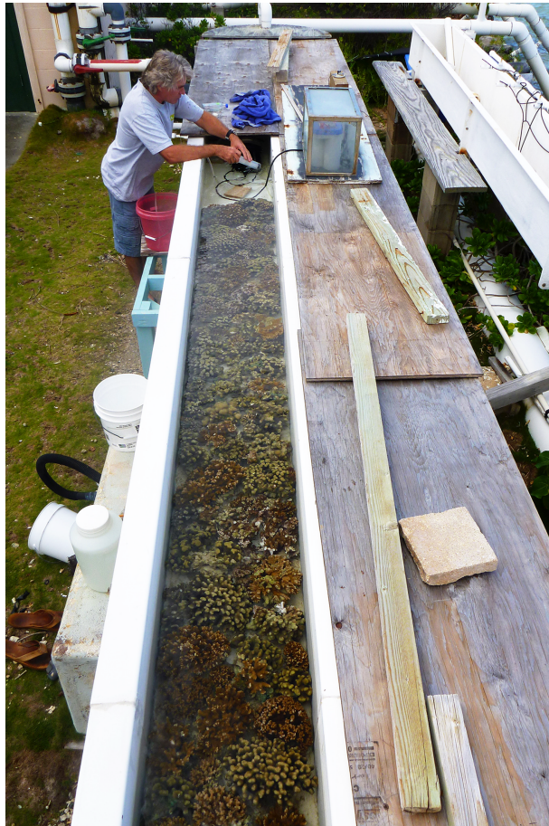
Figure 1 Flume system. The flume system with the shade cloths taken off showing the sub-sample bucket in use.
