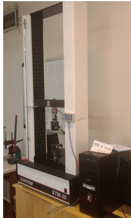
Fig. 3 Santum-STM 20, UTM prior to application of dislodging force
