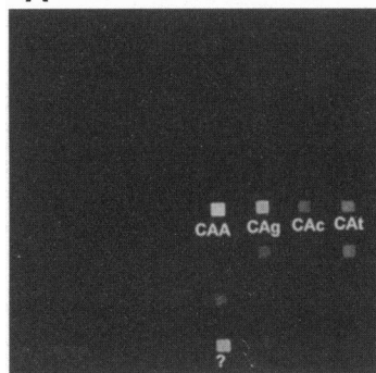
FIG. 2. The effect of mismatches in different positions of the duplex on hybridization efficiency. A 2.2 \times 2.2-mm microchip (100 \times 100 \times 20 \mu m gel elements, see Fig. 1) contains 64 immobilized octamers with all four bases in the three 5'-terminal positions. The bases in these positions ( x , y , and z ) are indicated on axes x , y , and within proper squares z . The microchip was hybridized with HEX-5'-GTCCAGTT-3', a 8-mer fluorescently labeled at the 5'-terminal position. (A) Fluorescence microscope image. (B) Fluorescence intensities in arbitrary units. The terminal mismatches are indicated above the intensity columns. The ? shows unexpected strong signal from the duplex with T-T mismatch in preultimate position, which has not been observed in other experiments.
