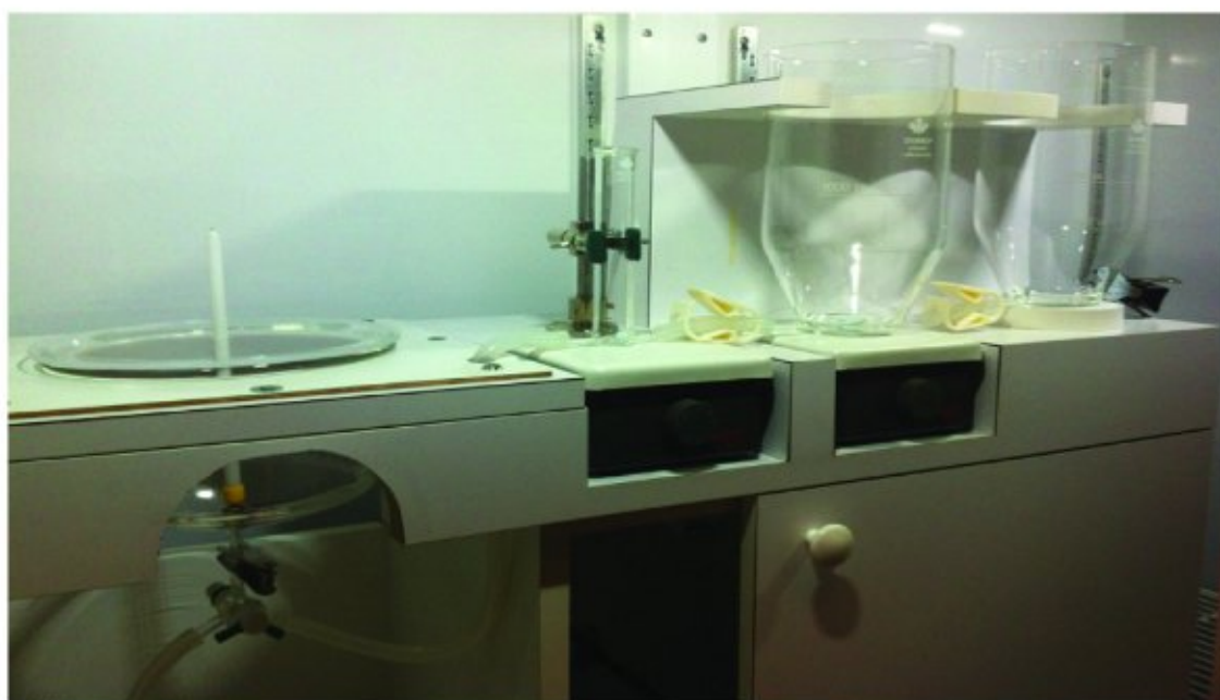
Figure 1. Setting up the STA-PUT Apparatus: A schematic and actual image of the STA-PUT apparatus are shown. All glassware is connected by plastic tubing, including the tube that connects the apparatus to the fraction collector. Arrows indicate location of clamps. A) Cell loading chamber, contains a stir bar; B) 2 L cylinder for 2% BSA, contains a stir bar; C) 2 L cylinder for 4% BSA; D) Sedimentation chamber; E) Stir plates; F) Baffle; G) Stopcock. Click here to view larger image.
