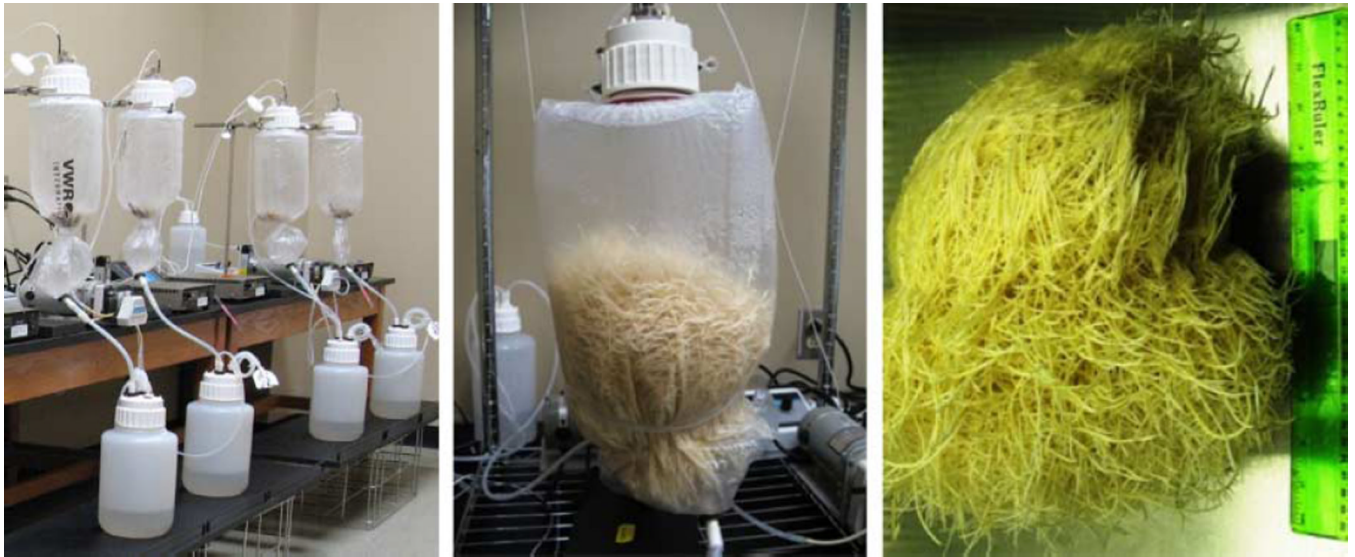
Figure 1. The mist reactor used in these studies. Left, a group of 4 L reactors with A. annua ; middle, 20 L reactor with A. hypogaea roots; right, A. hypogaea roots harvested from 20 L reactor (ruler = 30 cm).
