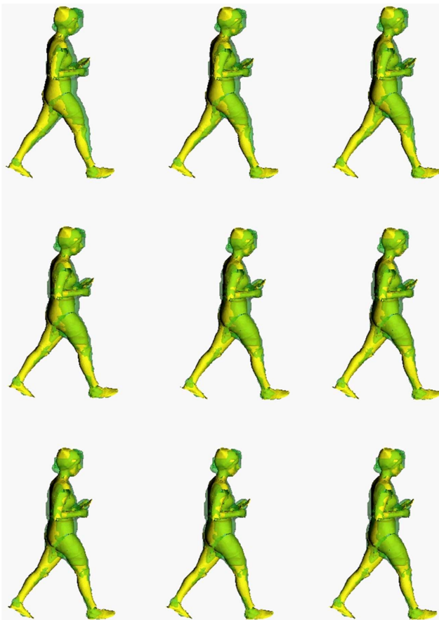
Figure 5. Example of nine iterations of the articulated-ICP algorithm for matching of the model (yellow) to visual hull data (green). doi:10.1371/journal.pone.0087640.g005
