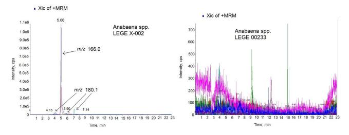
**Figure 7.** Positive multiple reaction monitoring (MRM) mode chromatogram and MS spectra of the 4.15 min peak, 5.90 min peak and 7.14 min peak from *Anabaena* spp. LEGE x-002 extract on the triple quadrupole mass spectrometer (QTRAP) instrument. Transitions monitored in the MRM method: m/z 180.1 > 180.1, m/z 180.1 > 163; m/z 180.1 > 145.0, m/z 180.1 > 68, m/z 180.1 > 43. The precursor ion in the MS2 mode: m/z 180.1. Collision Energy (CE): 30.
