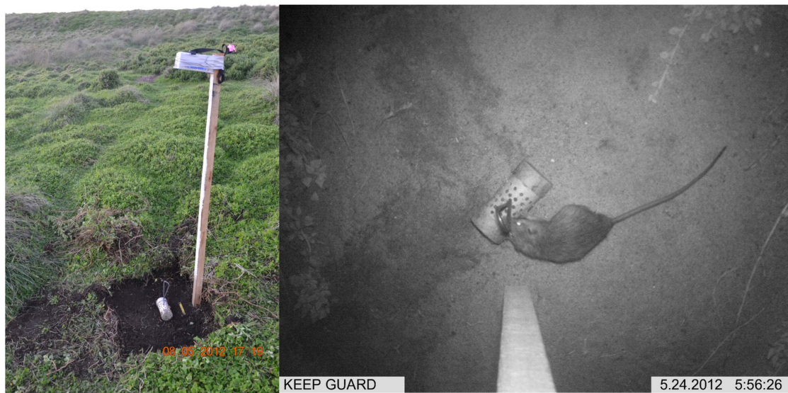
Figure 1. The set-up of the camera traps used in this research. Horizontal mounting setup demonstrating how the camera provides a 'birds-eye view' of the bait lure (left). Image of a black rat (right) demonstrating the type of images obtained, and the ease of identifying key features (tail length, ear morphology).
