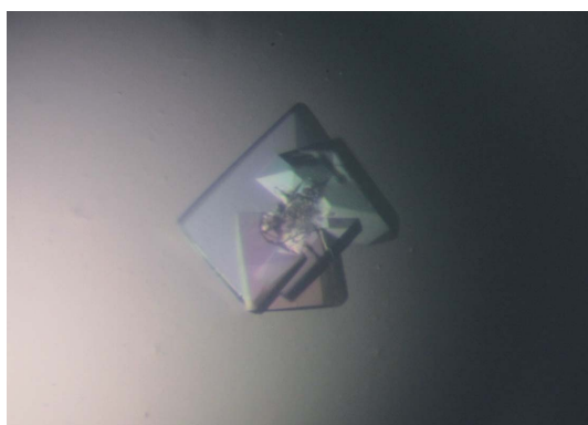
Figure 2 Crystals of IL3R \alpha –CSL362 grown by vapour diffusion at 22°C in a mother liquor consisting of 22% PEG 3350, 200 mM sodium malonate, 100 mM citrate buffer pH 6.4. The larger crystal in the centre of the picture is approximately 0.03 \times 0.1 \times 0.1 mm in size.
