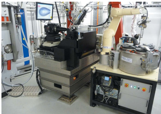
Figure 1 Experimental endstation of beamline X10SA. From left to right: Pilatus 6M area detector (Dectris), D3 diffractometer, CATS robotic sample changer system (IRELEC).
