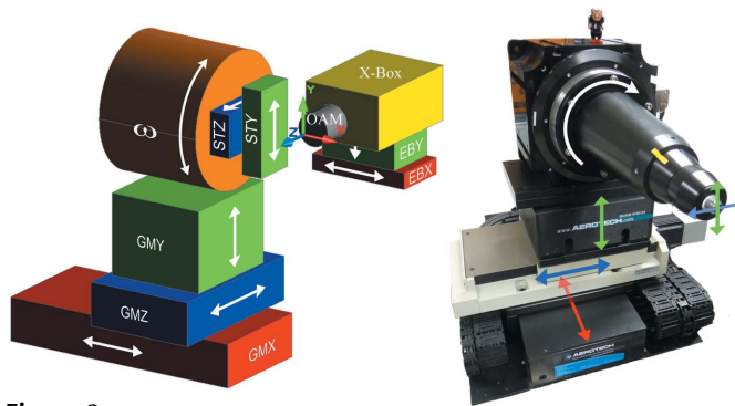
Figure 2 Left: degrees of freedom (DOF) of the D3 diffractometer. The translations GMX, STY and STZ and the rotation \omega are used for scanning operations, i.e. with the X-ray shutter opened, the translations GMY and GMZ are used for sample positioning during alignment only. The active X-ray beam feedback to an X-ray beam-position monitor in the so-called exposure box (X-Box) allows the positioning of the beam via the EBX and EBY translations. The on-axis microscope is the reference device to which all others are aligned; the sole DOF with a relation to the microscope is the GMZ translation of the goniometer that is used to bring the sample into focus. Right: DOF mapped onto the actual goniometer.
