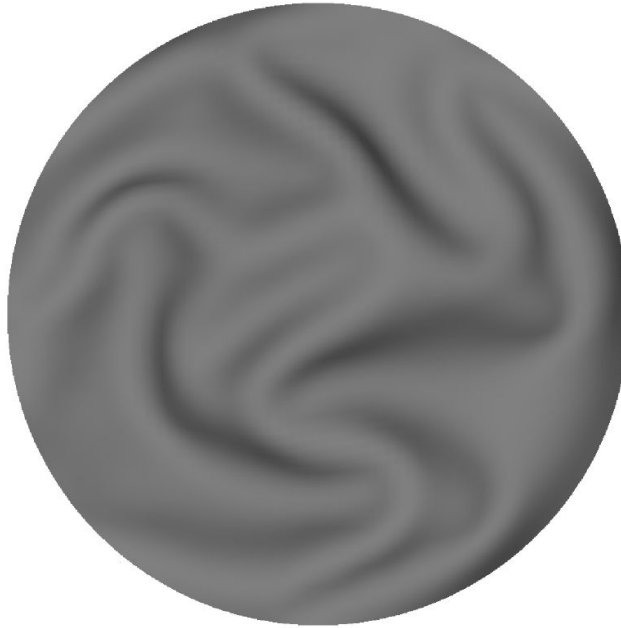
Figure 3. Top view of the membrane deformed configuration at t = 0.15 s. Despite the complex deformation pattern, the wrinkles on the membrane surface are smooth.
