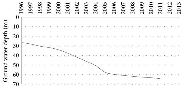
FIGURE 1: Groundwater depletion in Dhaka City [1].
