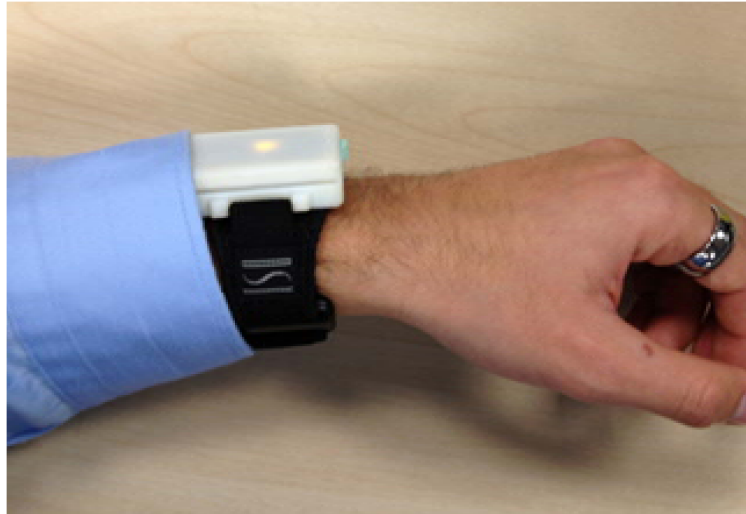
Fig. 1. The manometer consists of a sensing and data-logging board worn in a watch-like enclosure and a magnetic ring worn on the finger. The device senses wrist flexion/extension, wrist deviation, finger flexion/extension, and gross arm movement
