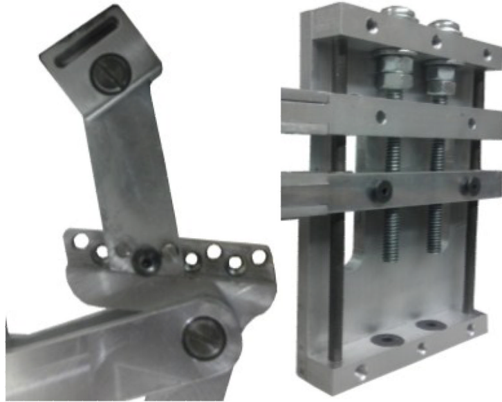
Figure 2. Finger size adjustment of the proximal phalanx (left) and vertical adjustment of the 8-bar mechanisms for the middle and index fingers (right).
