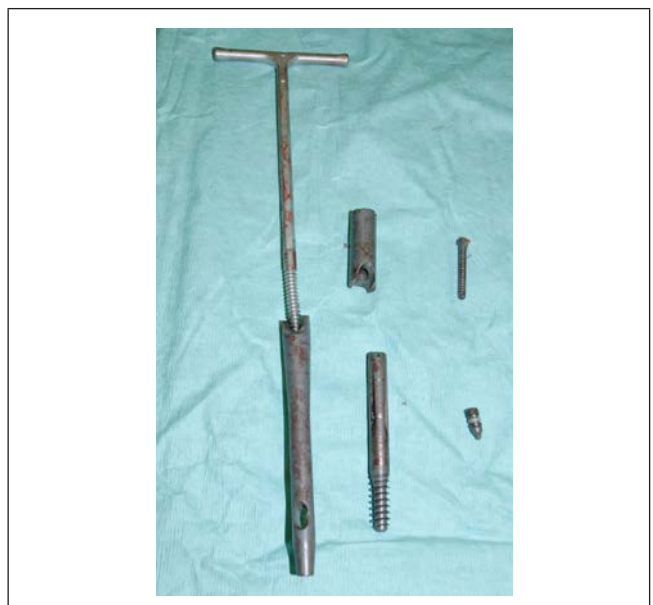
Figure 1 Corkscrew and distal fragment construct with (clockwise from top left) proximal fragment, distal locking bolt, set screw and lag screw
