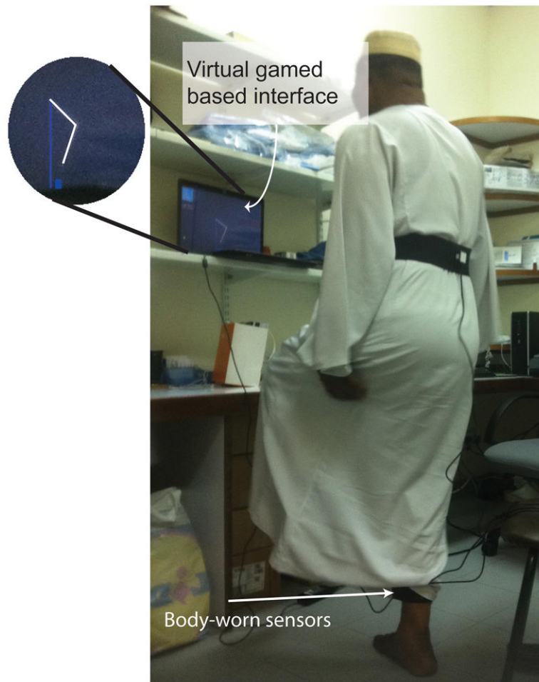
Figure 2. Protocol of test. Participants were presented with a virtual interface on a laptop screen placed in front of them. Their lower extremities were represented as a stick model in the center of the screen with the body facing the right side of screen
