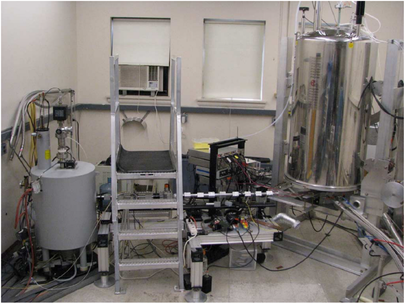
Fig. 9. Photo of the 250 GHz gyrotron oscillator (left), the 380 MHz NMR spectrometer (right).
