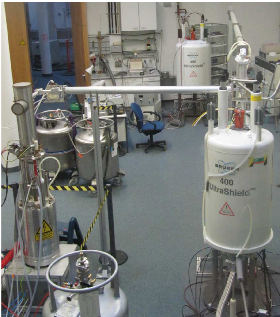
Fig. 13. 260 GHz Gyrotron Oscillator (left), with overmoded transmission line coupling the THz radiation to the NMR spectrometer (right). Photo courtesy of T. Prisner.
