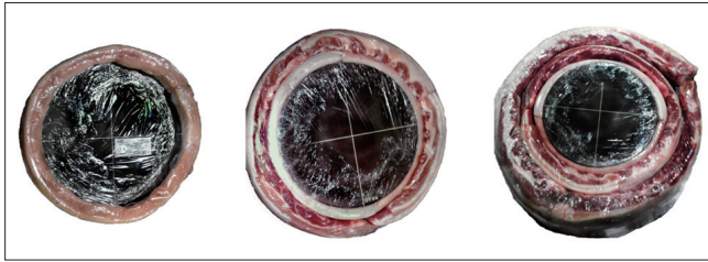
Fig. 1. Images of three phantoms with different thicknesses of subcutaneous fat: 24-cm-diameter phantom (left); 30-cm-diameter phantom (middle); and 40-cm-diameter phantom (right).
