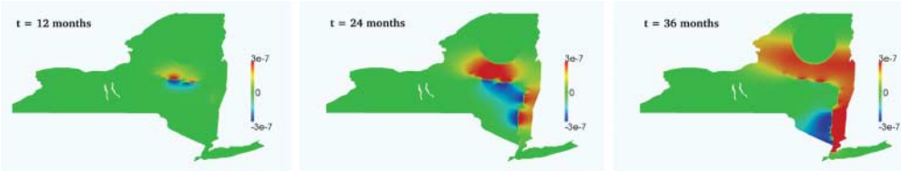
Figure 6. Effect of diffusion reduction normal to the river on the propagation front at (left to right) 12, 24, and 36 months: I_{base} - I_t .
