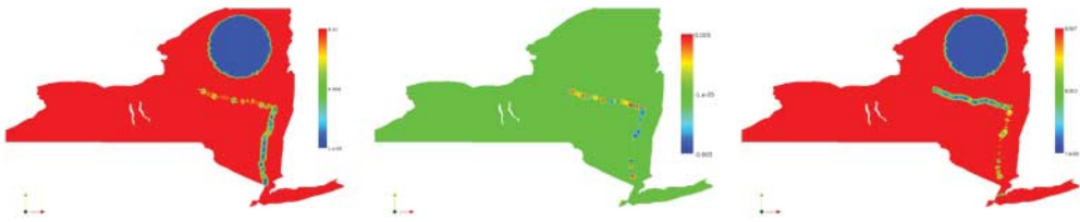
Figure 3. Left to right: diffusion in the x -direction, cross-diffusion, and diffusion in the y -direction ( v_H = 0.01 , v_L = 5 \times 10^{-3} \times v_H ).
