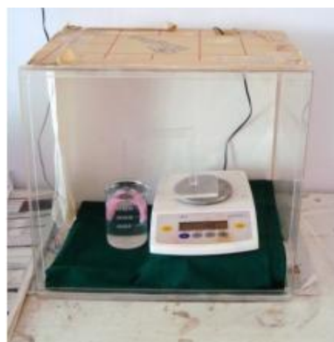
Figure 8: Weighing Whole Denture Base in Water.
