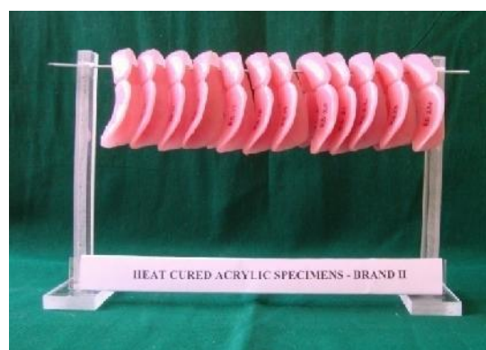
Figure 7: Heat Cured Acralyn H Specimens.
