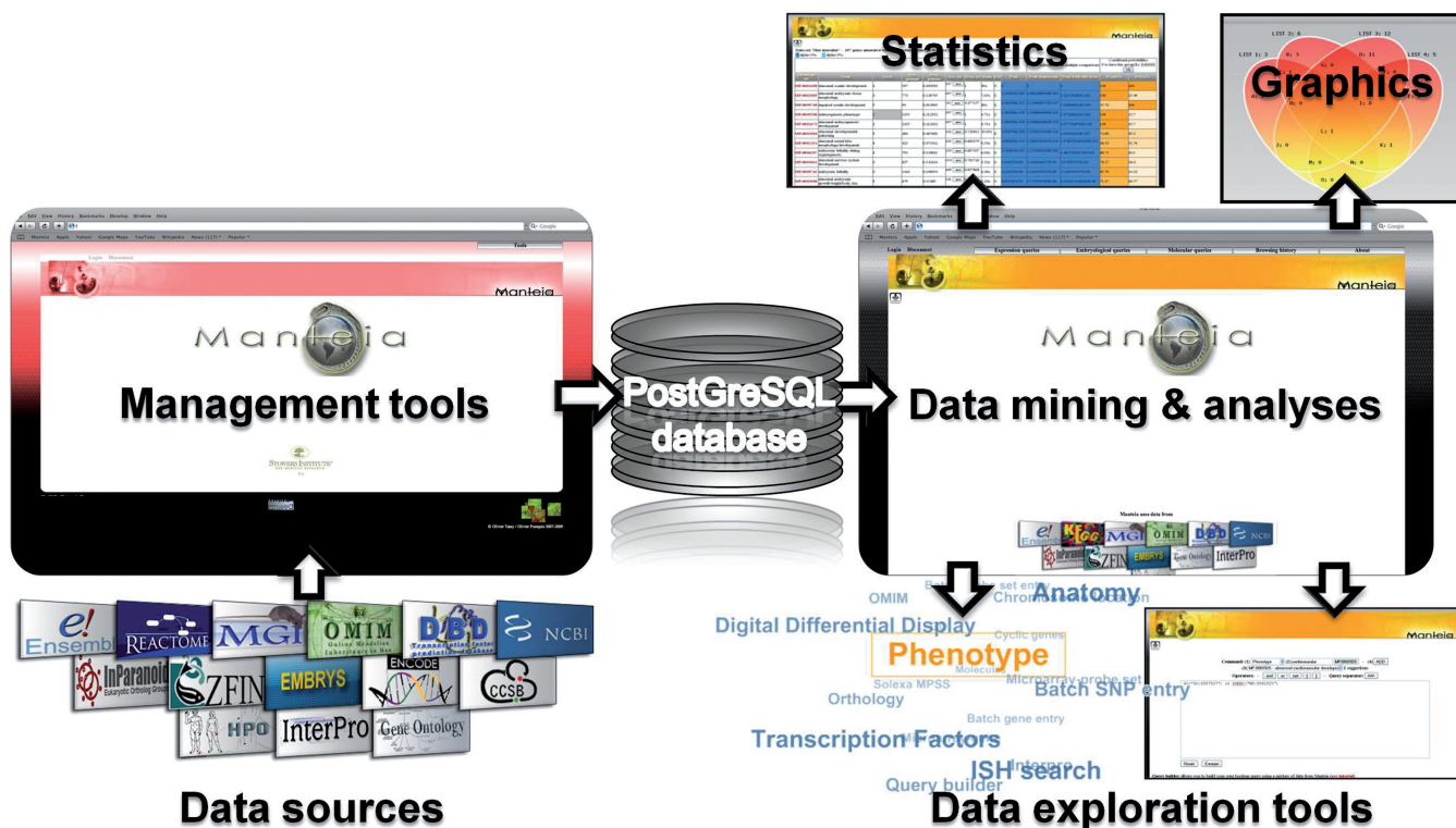
Figure 1. Overview of the Manteia architecture. Data are collected from various databases for several species. They are then processed by the management tools and accessed with the online user interface. Over 30 exploration, graphical representation and statistical tools are available. All the tools are interoperable, which makes it possible to analyze the information, perform data mining and make predictions.
