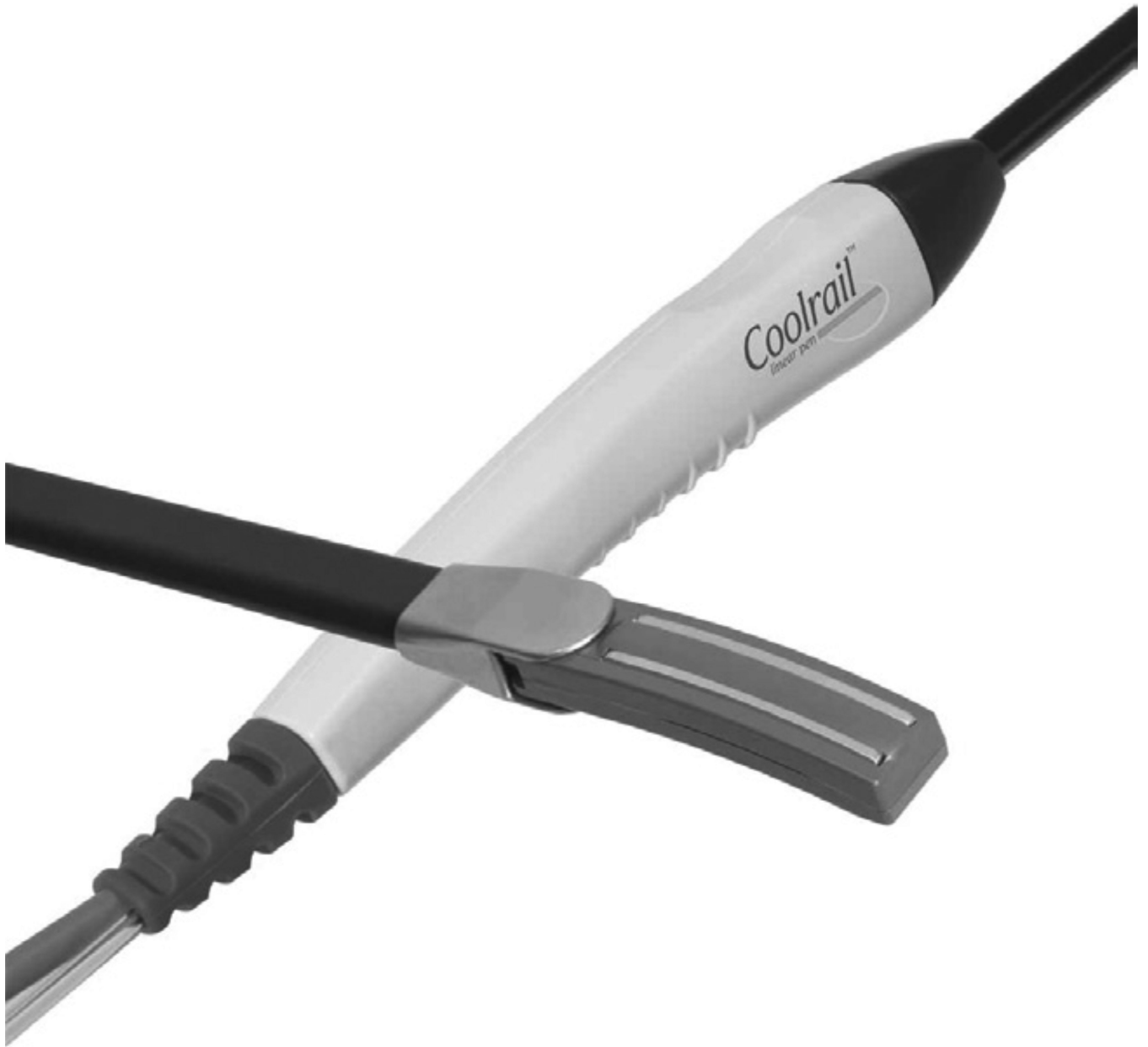
Figure 2. The AtriCure Coolrail device. The two electrodes are hollow and sterile water is circulated internally to provide cooling of the electrode-tissue interface during ablation. They are 3mm wide and 30mm long.
