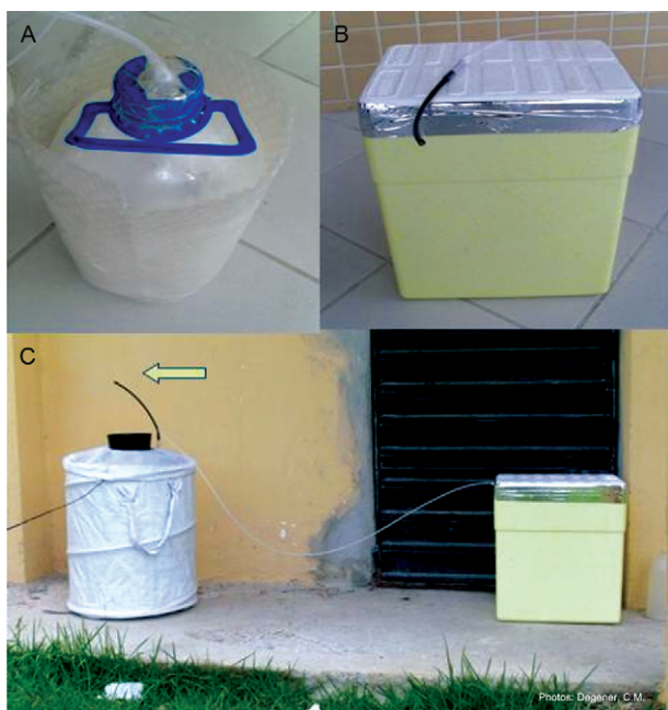
A: filled PET-bottle with 3 Kg of dry ice and carbon dioxide (CO 2 )-nozzle, surrounded by bubble foil; B: sealed 20L-Styrofoam box with CO 2 -nozzle; C: BG-Sentinel® trap with CO 2 -nozzle (arrow) which is connected by a plastic tube to the dry ice-filled PET-bottle.
