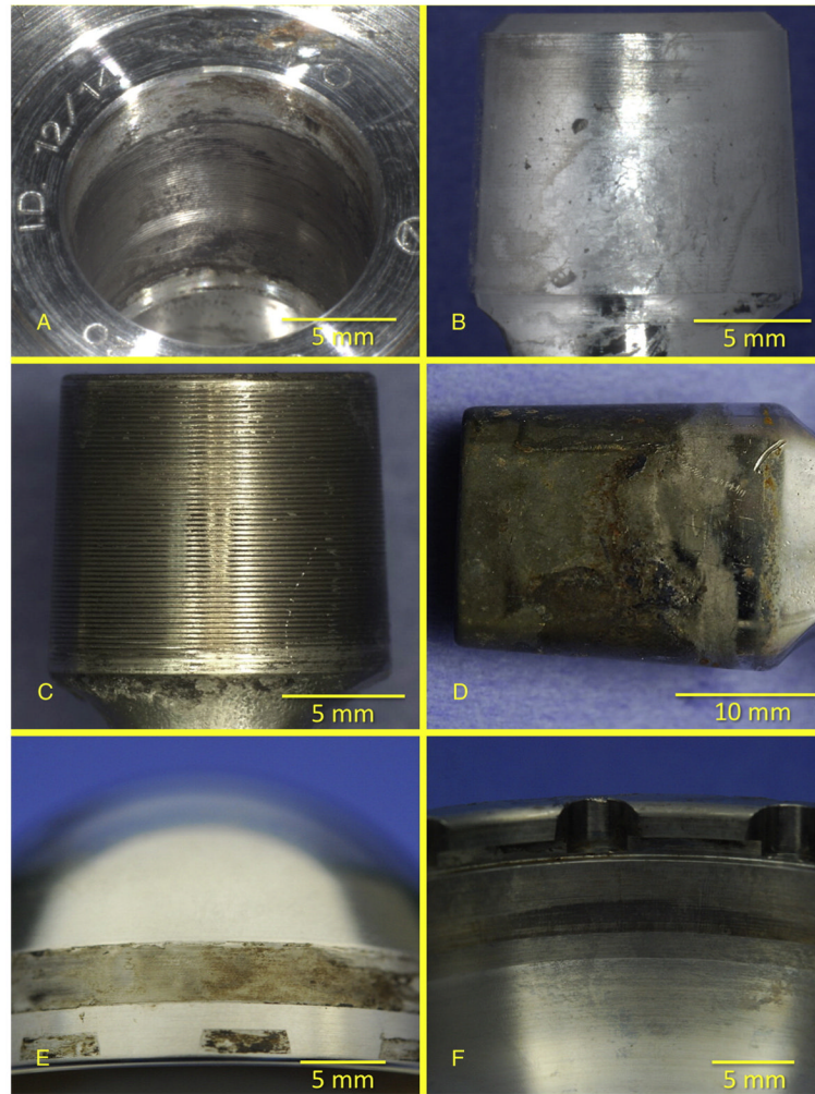
Fig. 1. Photographs showing examples of modular interface damage on components in this study. (A) head taper, 4. (B) stem taper–monolithic stem, 3. (C) stem taper–modular neck, 4. (D) distal taper of modular neck, 4. (E) backside of modular liner, 4. (F) mating surface of modular shell, 2.
