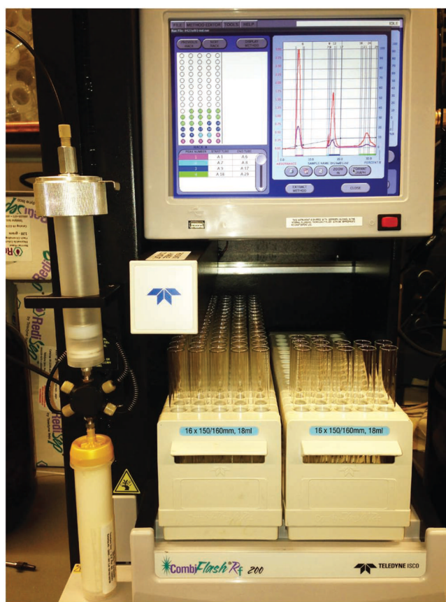
Figure 8. Separation of reaction mixture by flash column chromatography.
