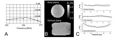
**FIGURE 2.** Parameters of AG/LGR. A. Isolation. Markers show 20 MHz frequency range and the center frequency. B.  $B_1$  maps of AG/LGR as measured by Rabi nutation imaging. C.  $B_1$  along three directions passing the geometric center of a resonator. Solid circles mark  $B_1$  of the standalone AGR, while open circles mark AG/LGR.
