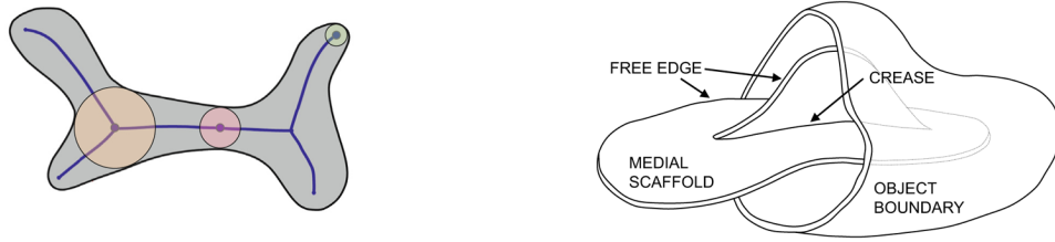
Fig. 1. Left: the medial axis of a 2D object, with examples of MIBs tangent to the boundary at one, two and three points. Right: an illustration of a 3D object, half of which has been cut away to reveal the medial scaffold. The medial scaffold consists of surface patches that join along crease curves and terminate at free edge curves.
