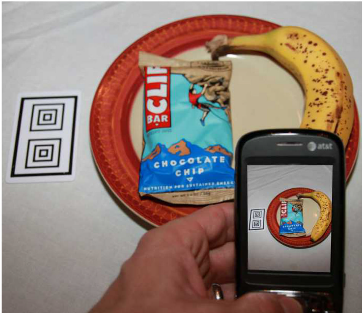
Figure 1. When using the RFPM, participants use a Smartphone to capture images of their food selection, plate waste, and a reference card. These images are then immediately sent to a server for analysis.
