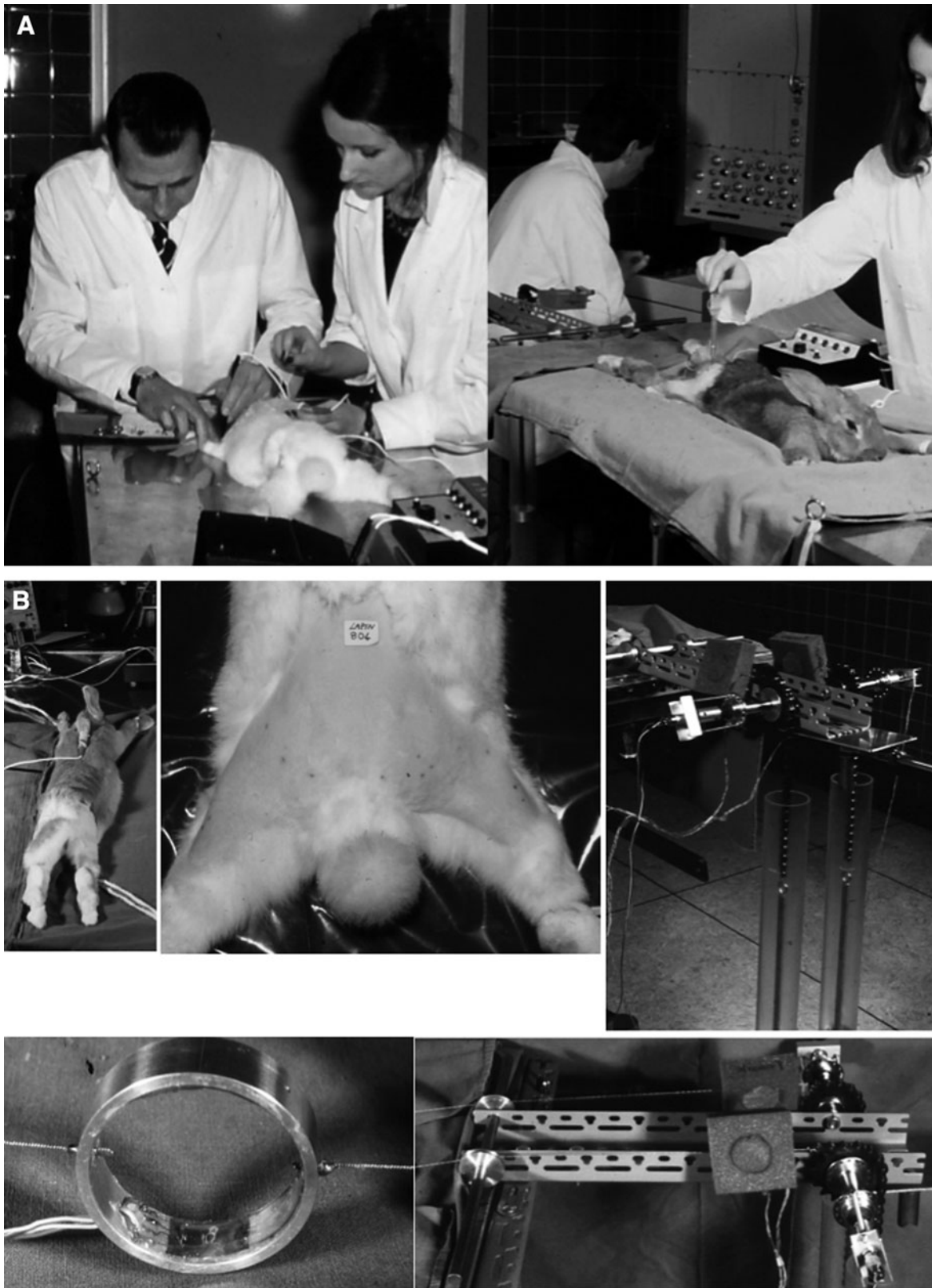
FIG. 4. Experimental model of analgesia on hind limbs of rabbit. (A) Insertion of acupuncture needles by Niboyet and Terral in two acupoints. (B) Measurement of the withdrawal reactions (reflex forces) with strain-gauge transducers. (C) Record of forces after painful puncture of skin with a detector equipped with strain gauges ( middle line ): on the left , before, and on the right , after 20 minutes of electrical stimulation of the two acupoints of the right hind limb (there were no more withdrawal reactions). (D) Implantation of a microelectrode into the nucleus parafascicularis of the thalamus of a rabbit with its head in a stereotactic frame. Bottom left shows pain signal recorded by the thalamic electrode during painful stimulation, and bottom right shows inhibition of pain signal after acupuncture stimulation.
